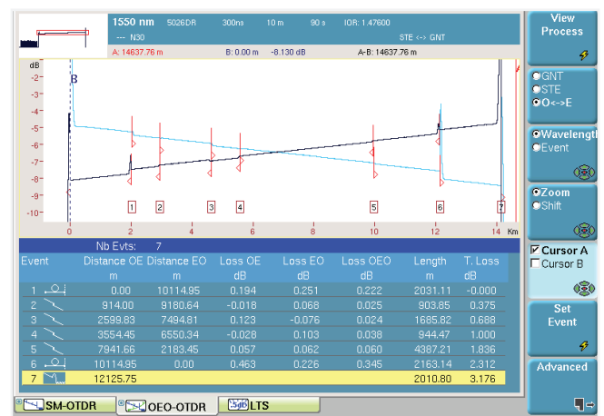
Figure 3. Bidirectional OTDR measurement
