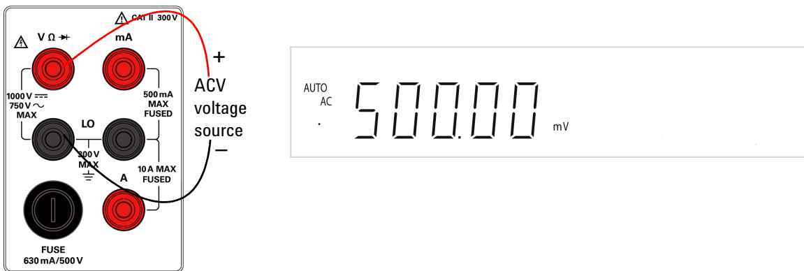
Figure 1-10 ACV terminal connection and display
