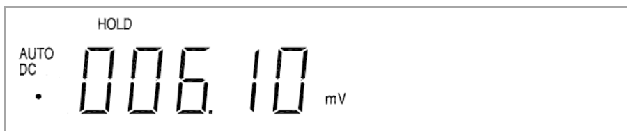
Figure 2-7 Typical refresh hold operation display
