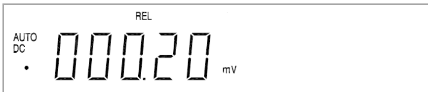
Figure 2-2 Typical Rel operation display
