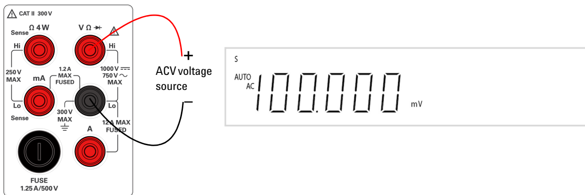
Figure 1-10 ACV terminal connection and display
