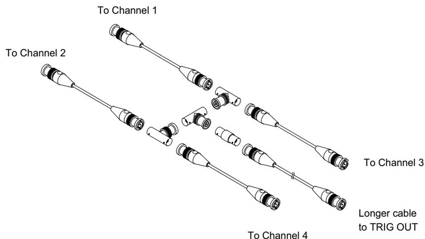
**Figure 51** User Calibration cable for 4-channel oscilloscope
