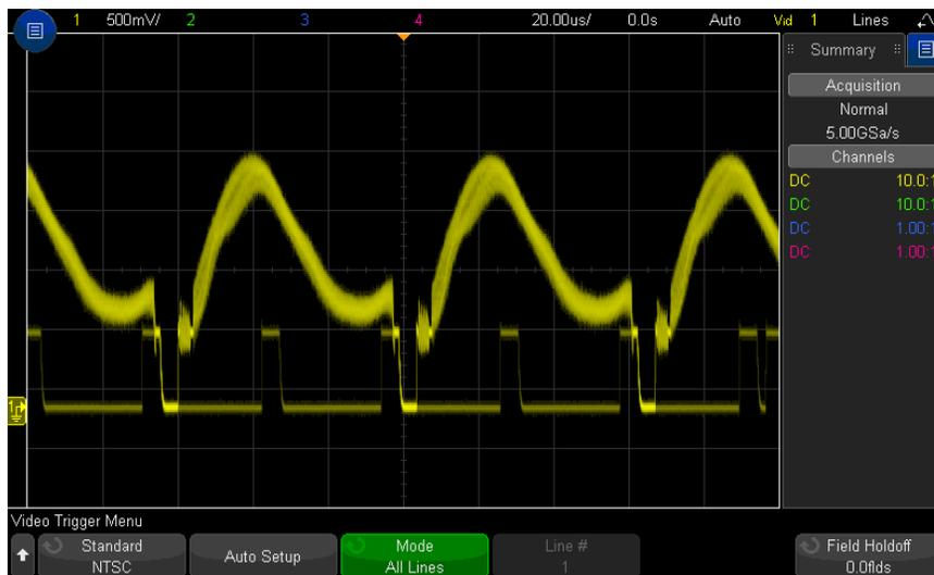
**Figure 29** Triggering on All Lines
