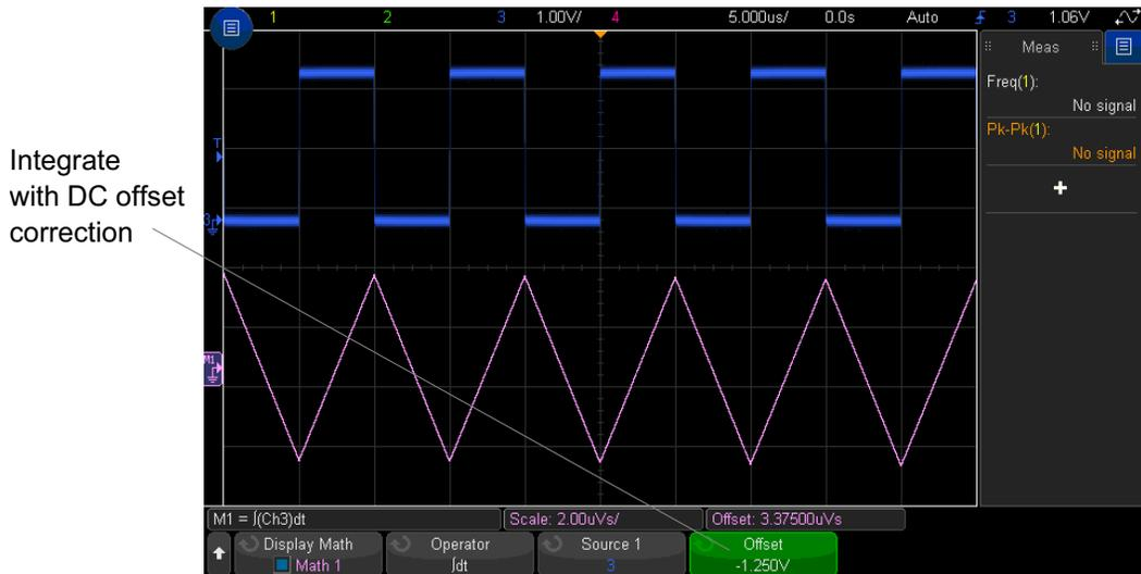
**Figure 10** Integrate With Signal Offset
