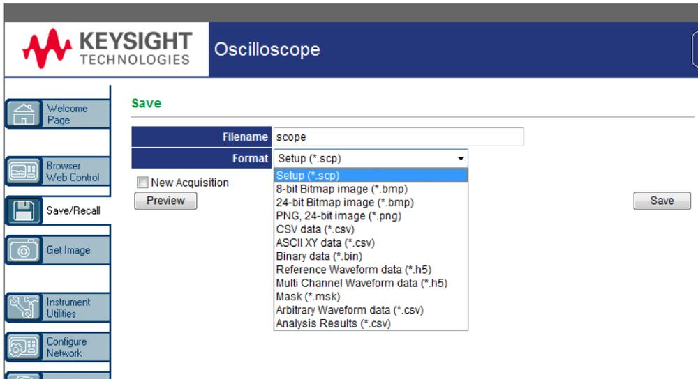
You can click **Preview** to view the oscilloscope's current screen image. When previewing, you can use the **New Acquisition** check box to force a new acquisition before the preview.
