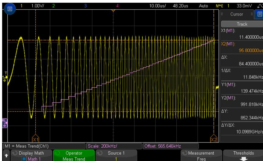
**Figure 18** Example of Measurement Trend
