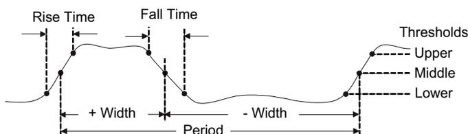
The default lower, middle, and upper measurement thresholds are 10%, 50%, and 90% between Top and Base values. See **"Measurement Thresholds"** on page 266 for other percentage threshold and absolute value threshold settings.
