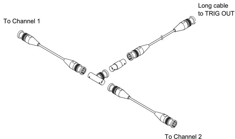
**Figure 50** User Calibration cable for 2-channel oscilloscope
