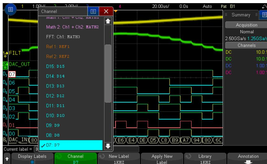
The figure above shows the list of channels and their default labels. The channel does not have to be turned on to have a label assigned to it.
