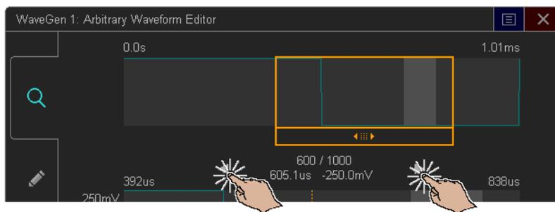
To adjust the value of a point, drag the voltage level handle up or down:
