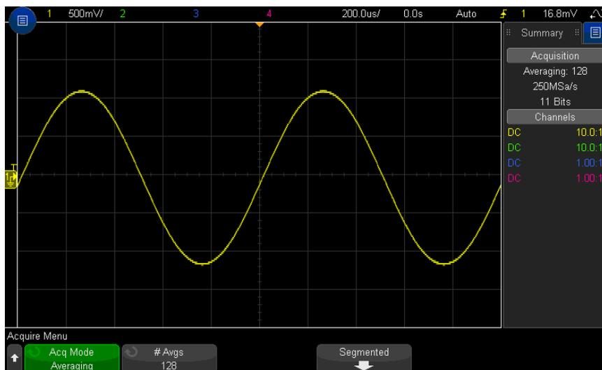
**Figure 40** 128 Averages used to reduce random noise
