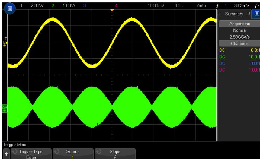
**Figure 26** Amplitude Modulation Shown at 100% Intensity
