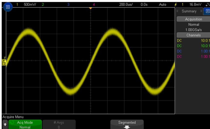
**Figure 39** Random noise on the displayed waveform
