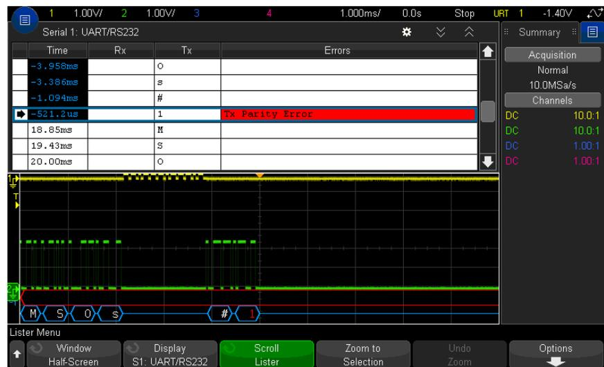
Before you can select a row or navigate through the Lister data, oscilloscope acquisitions must be stopped.
