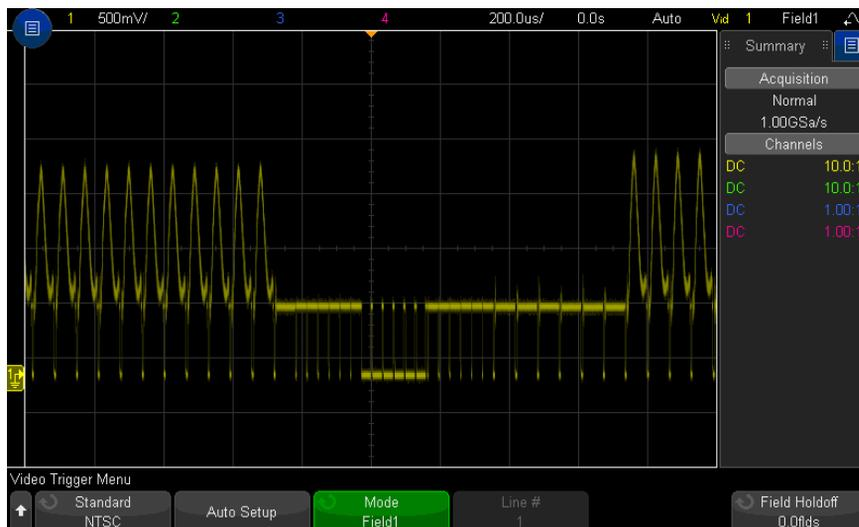
**Figure 30** Triggering on Field 1
