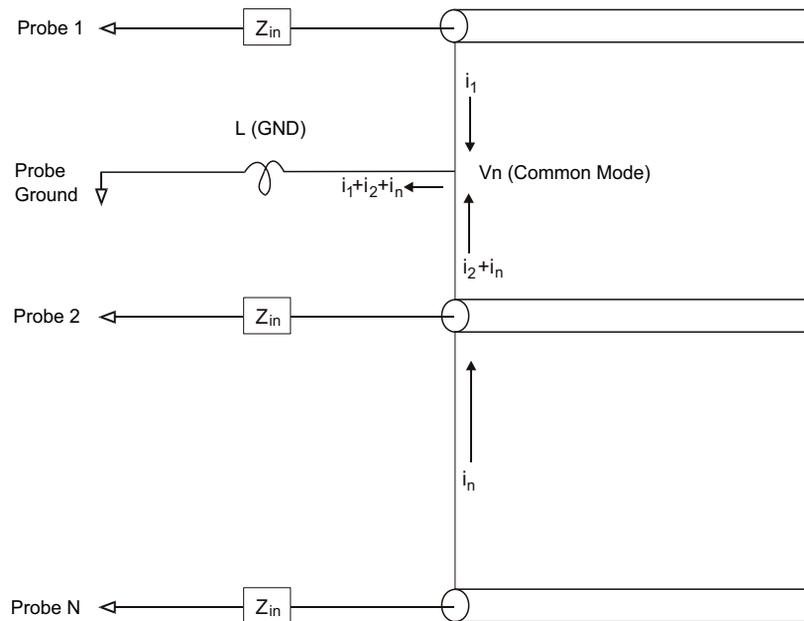
**Figure 25** Common Mode Input Voltage Model
