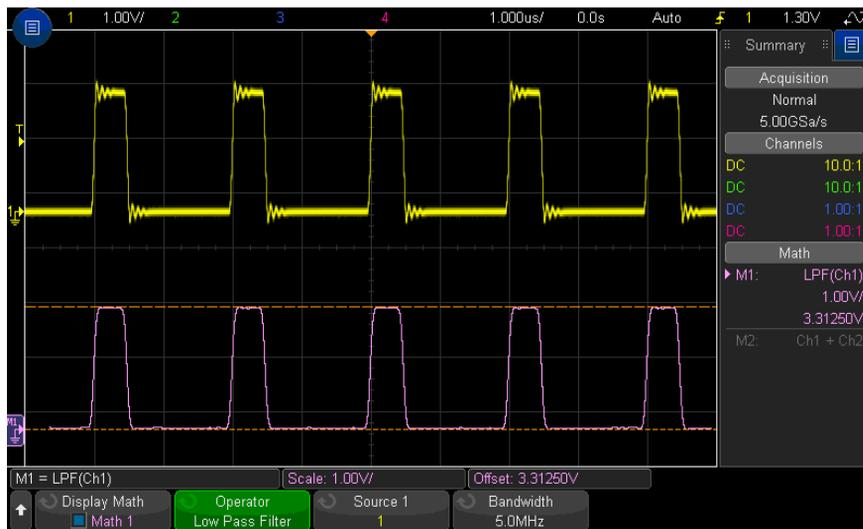
**Figure 16** Example of Low Pass Filter
