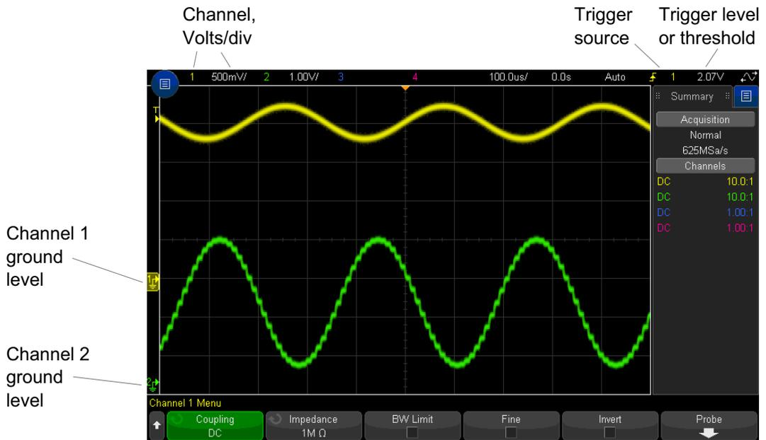
The ground level of the signal for each displayed analog channel is identified by the position of the
