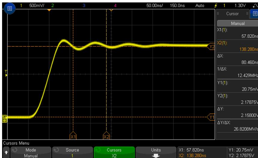
**Figure 42** Cursors measure frequency of pulse ringing
