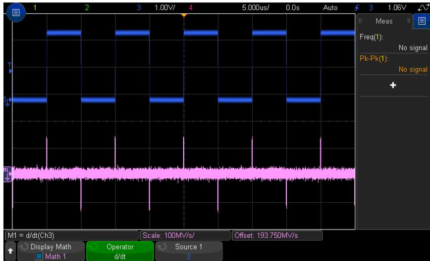
**Figure 8** Example of Differentiate Function
