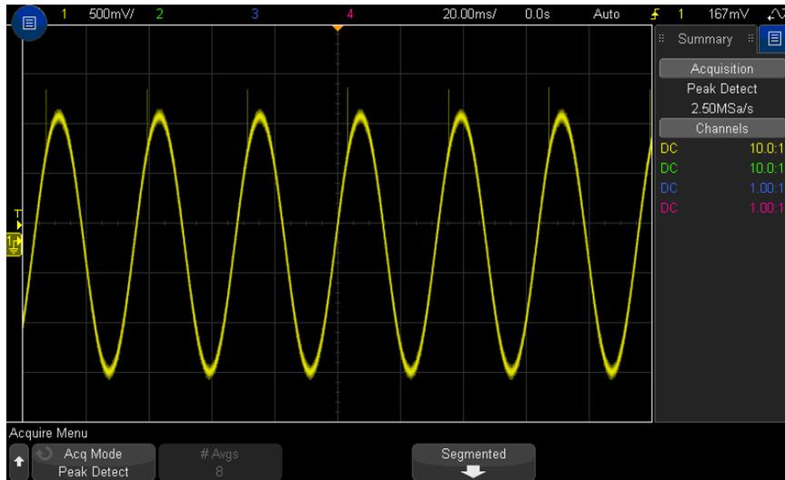
**Figure 38** Sine With Glitch, Peak Detect Mode
