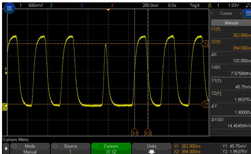
**Figure 44** Measuring pulse width with cursors
