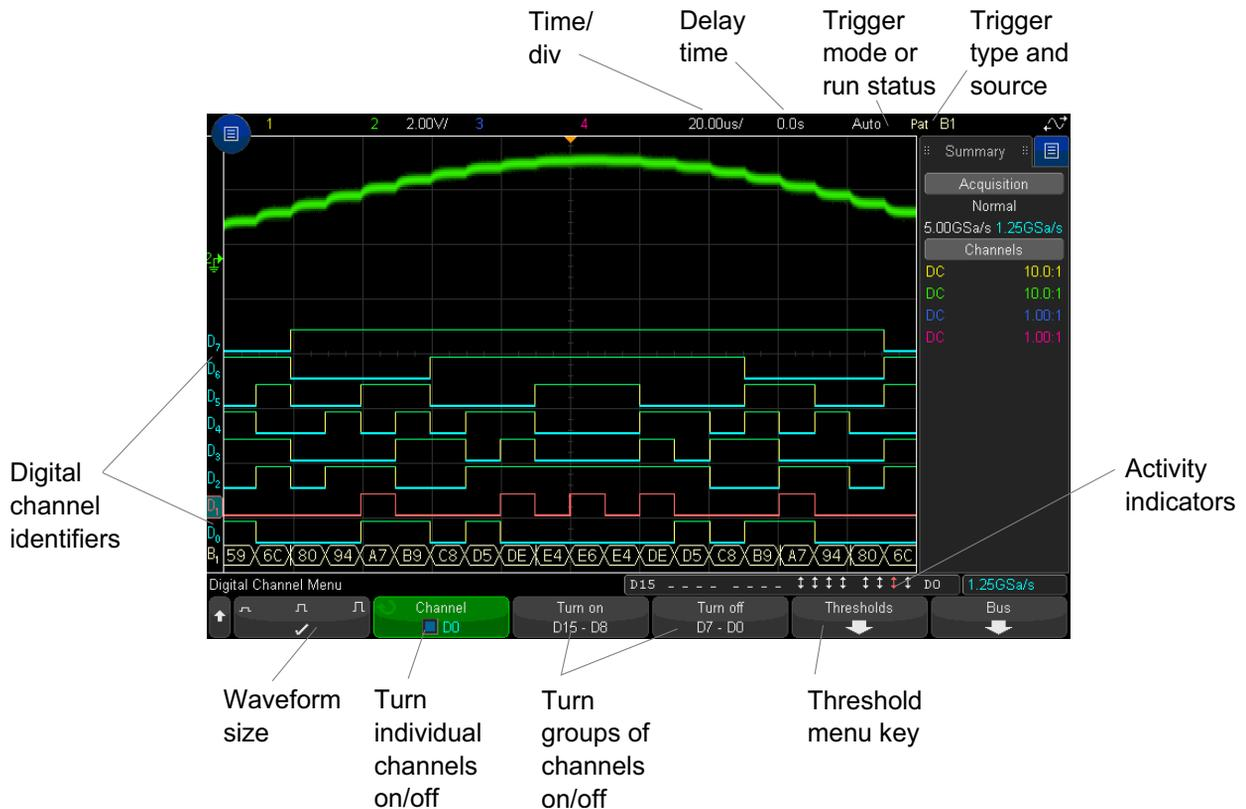
**Activity indicator** When any digital channels are turned on, an activity indicator is displayed in the status line at the bottom of the display. A digital channel can be always high (■), always low (■), or actively toggling logic states (⬆).
