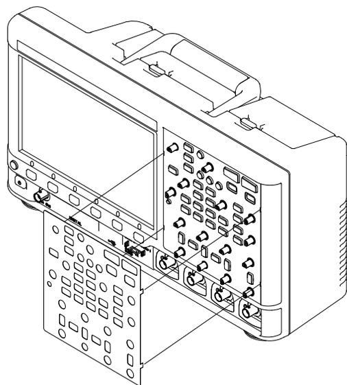
**3** Reinstall the front panel knobs.
