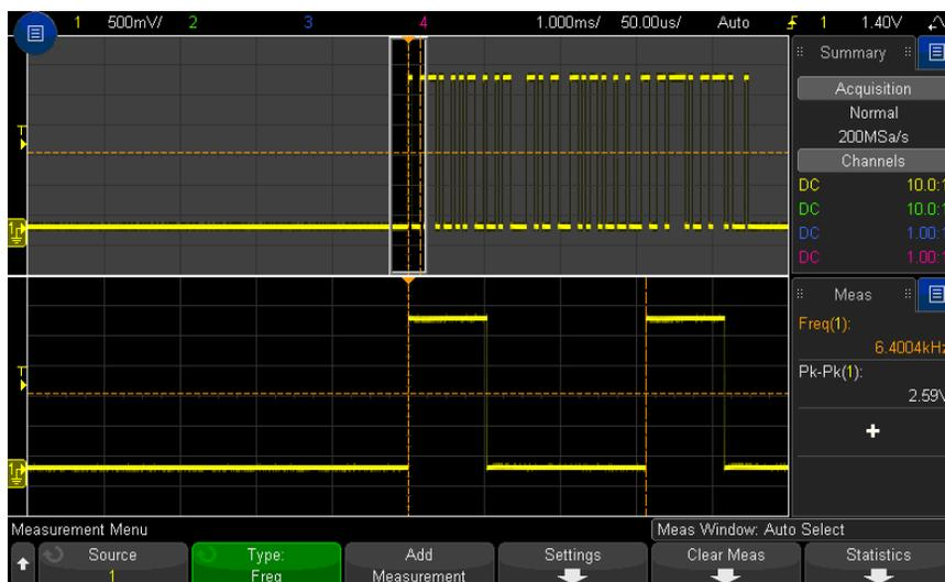
**Figure 49** Isolating an event for Frequency measurement
