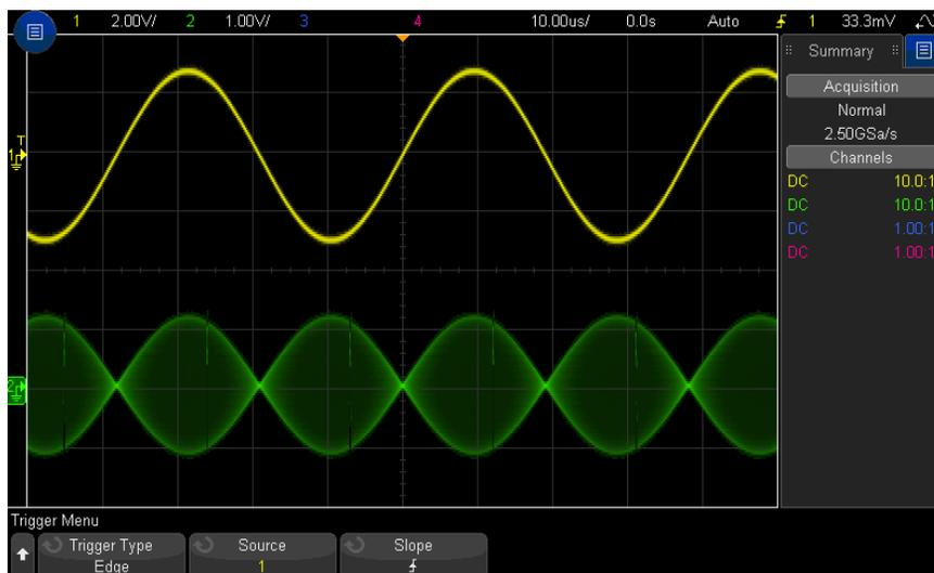
**Figure 27** Amplitude Modulation Shown at 40% Intensity
