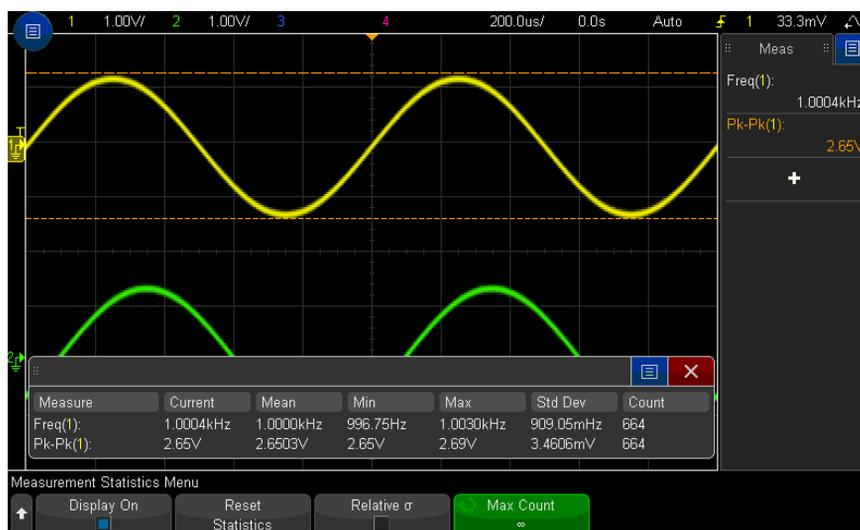
The source channel of the measurement is shown in parenthesis after the measurement name. For example: "**Freq(1)**" indicates a frequency measurement on channel 1.
