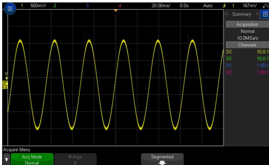
**Figure 37** Sine With Glitch, Normal Mode
