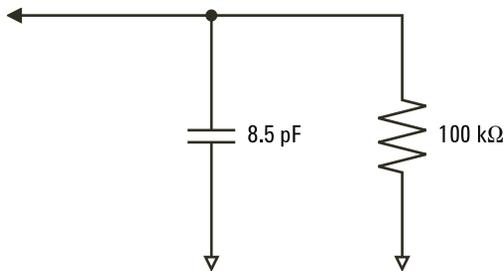
**Figure 22** DC and Low-Frequency Probe Equivalent Circuit
