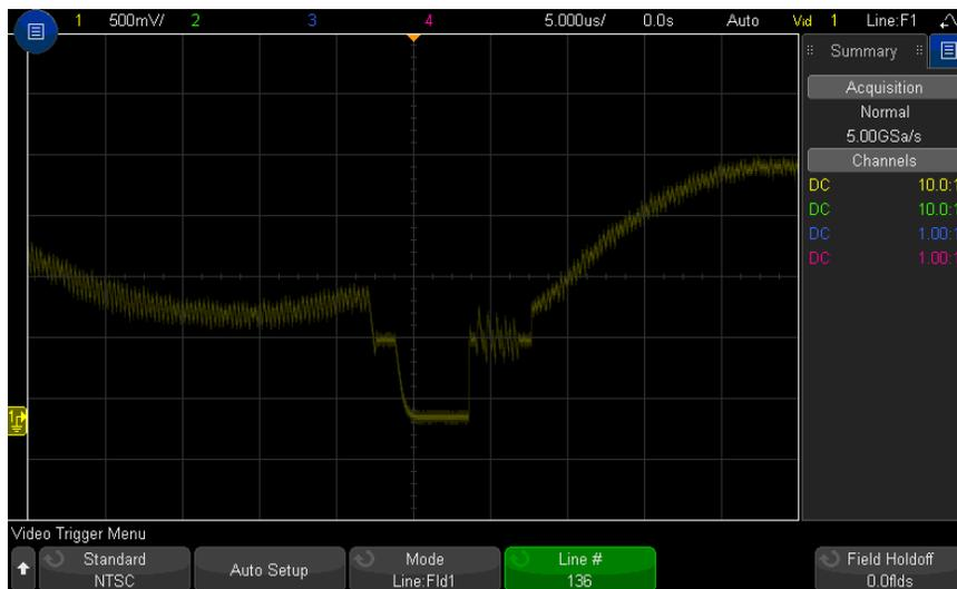
**Figure 28** Example: Triggering on Line 136
