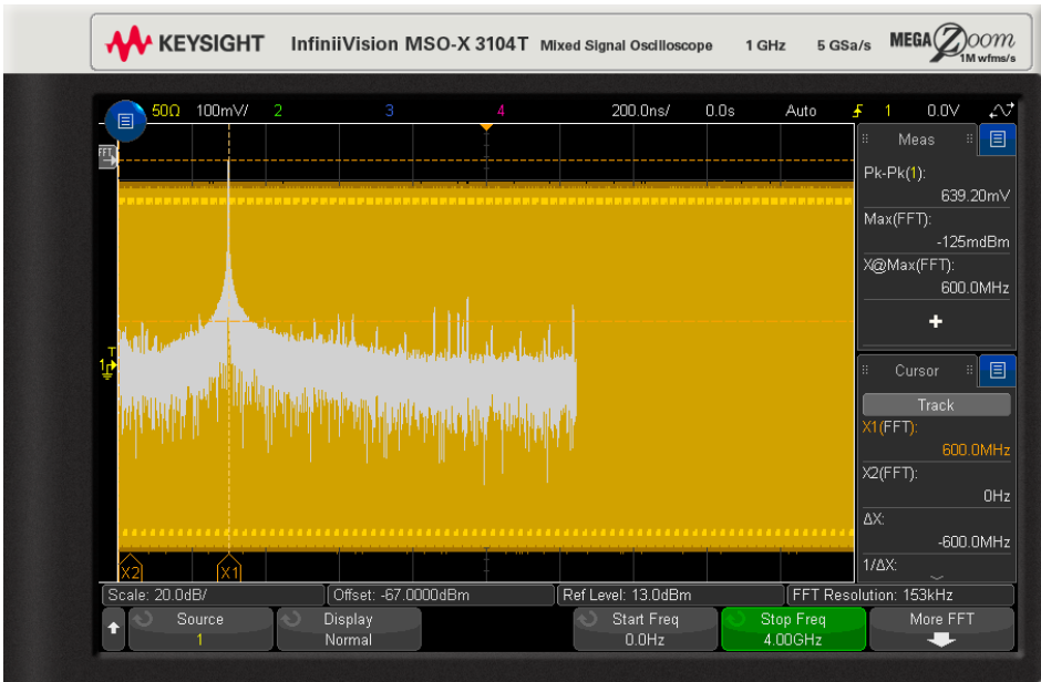
Figure 1. Time domain capture at 200 nsec/div and resultant FFT calculation with a 600 MHz sine wave input.
