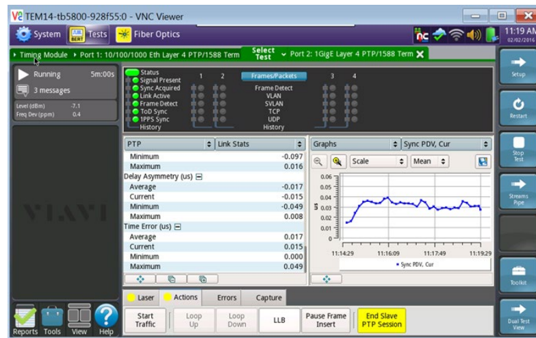
Figure 12. IEEE 1588v2 PTP test results
