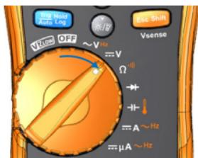
To power ON your multimeter, turn the rotary switch to any other position.
