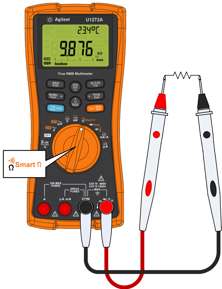
Figure 2-14 Measuring resistance
