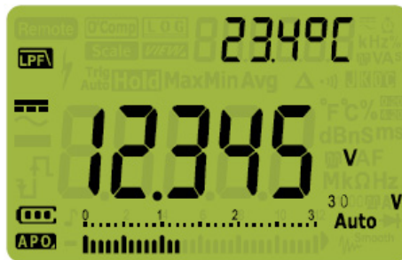
Figure 2-6 Filter for DC voltage measurements
