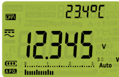
Figure 2-8 Low Pass Filter(LPF) for AC+DC voltage measurements
