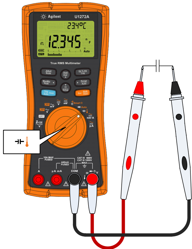
Figure 2-26 Measuring capacitance
