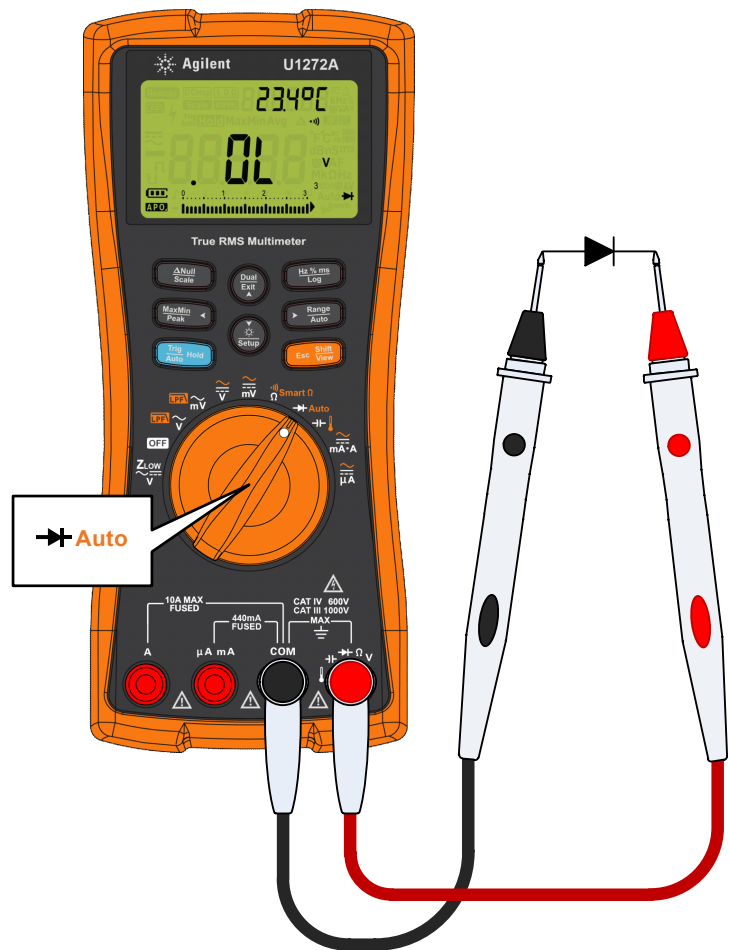
Figure 2-22 Testing reverse bias diode
