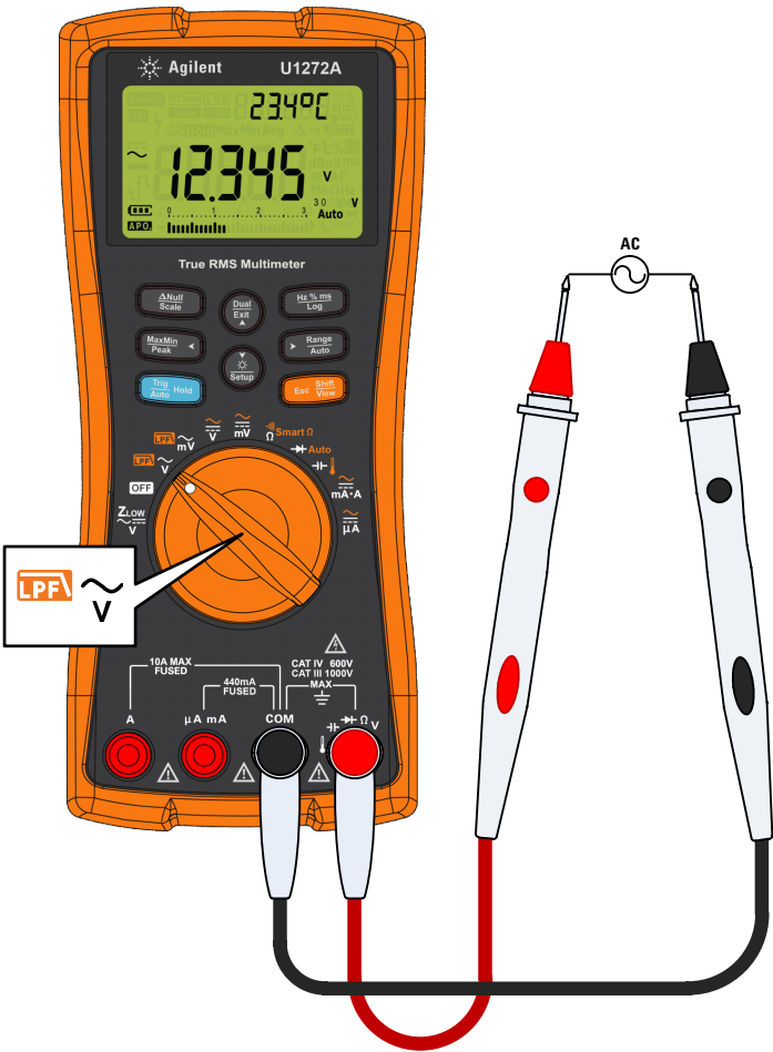
Figure 2-2 Measuring AC voltage
