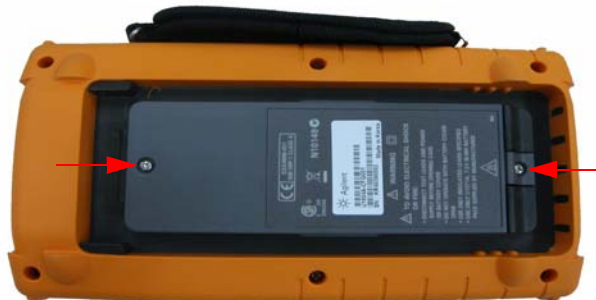
Figure 8-3 Remove battery cover screw
