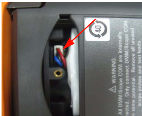
Figure 8-6 Unplug 2-wire connector with a tweezers.
