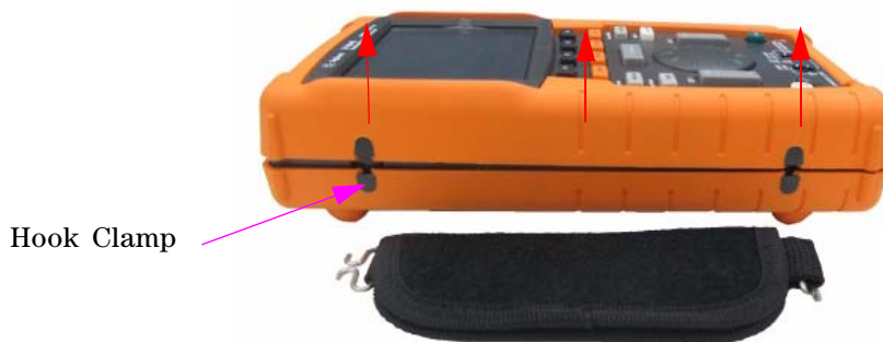
Figure 8-8 Remove handler from the instrument
