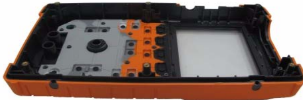
Figure 8-12 Remove keypad from the front cover
