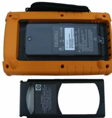
Figure 8-2 Disassemble the stand from the instrument
