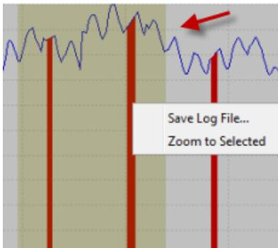
2. The network characteristics data is stored in a log file with the extension, .anr. The log file is essential in the next section, when the recorded network characteristics are played back in the lab.
