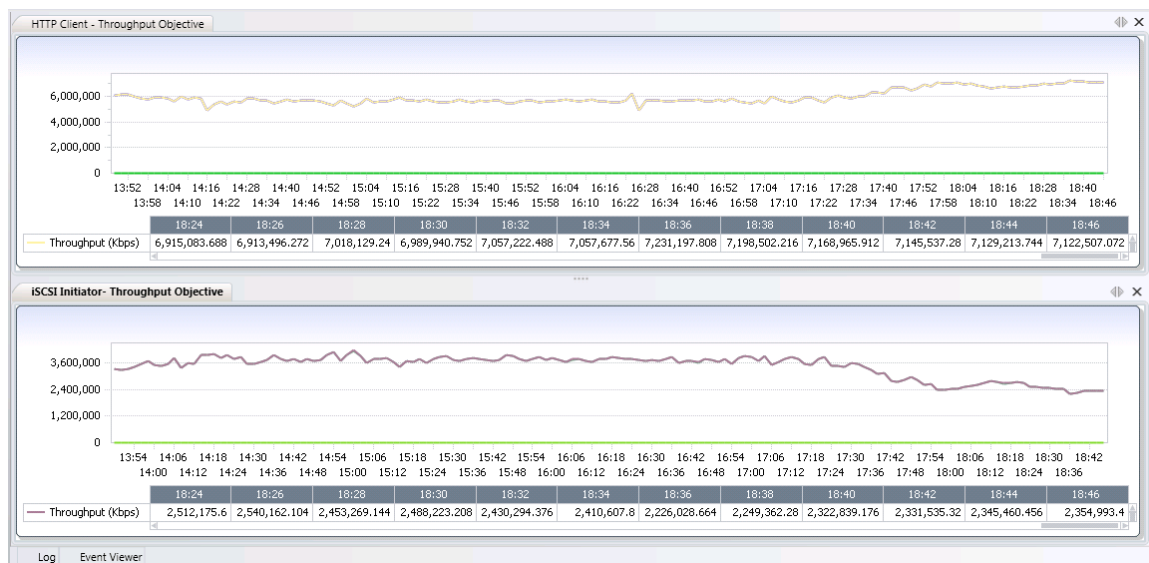
Figure 420. The throughput distribution with both HTTP and Storage traffic is not unpredictable and jittery.
