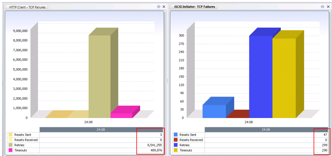
Figure 411. HTTP and iSCSI TCP Failures stat comparison shows that while HTTP had over 8Million retries the iSCSI has only 300 retries.
