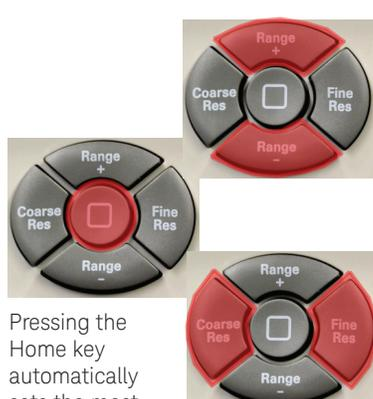
Pressing the Home key automatically sets the most appropriate range and speed at any time
