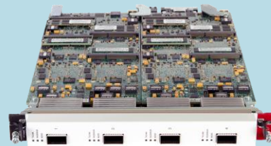
World's first Native CFP4 100GbE test module: Xcellon-Multis native CFP4 4x100GbE, 1-slot load module
