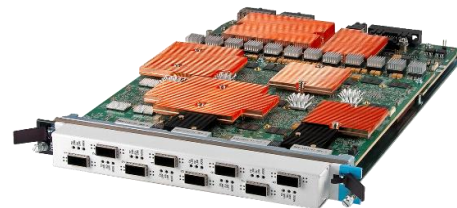
Novus and Novus-R native QSFP28 8-ports, 100/25 GbE, 1-slot load module
